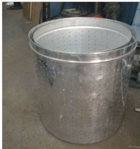
Figure 2: the 2nd chamber is placed inside the air treatment chamber.
