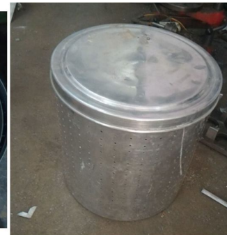
Figure 5: the air treatment chamber is closed using a lid.
