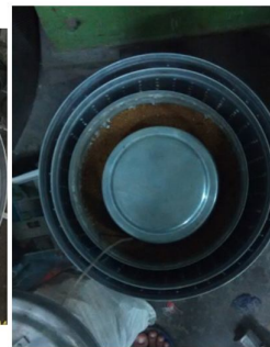
Figure 4: The vessel carrying the food item that needs to be protected from moisture is kept inside the chamber.
